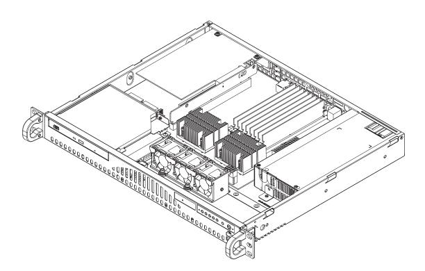
Figure 6-2. System Cooling Fans
